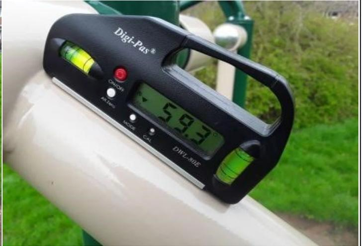
**Finding:** The swinging movement of the item exceeds the degrees from the vertical required by BS EN 16630 (59.3 degrees measured)
